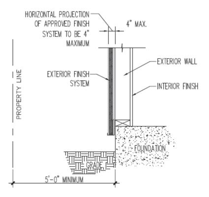
NOTE: INTERIOR AND EXTERIOR WALL FINISH SHALL CONTINUE TO FULL HEIGHT OF WALL.
